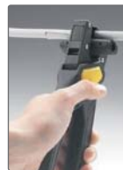
Round cut to the left and right of the longitudinal cut through 1/4 rotational movement of pliers
